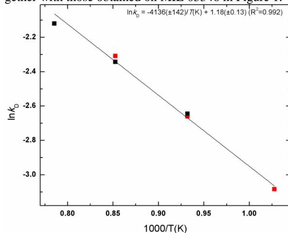
**Figure 1.**  $\ln k_D$  versus  $1000/T$  (K) for the augite samples considered in this work together with those by [4, 5]. Solid line represent geothermometer equation calibrated by linear fitting of MIL N.19 data (red squares) together with those obtained in this work (black squares).
